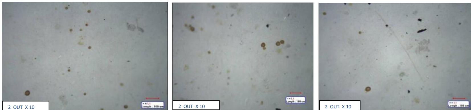
Effluents of the Spin Klin protected media filter(2). Time until CCM's \Delta p = 5m was 29:21 min.
